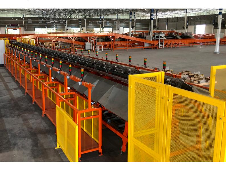
Denisort compact is a modular vertical sorter designed for the sortation of items with a weight of up to 12 kilograms. Total freedom in configuration and fast installation result in a powerful, compact and flexible system for maximum output on smallest footprint, perfectly tailored for a variety of applications, such as CEP services, e-commerce, retail, B2B and 3PL. The intended purpose of denisort compact includes the sortation for dispatch, goods in, returns, cross-docking and restmail.
