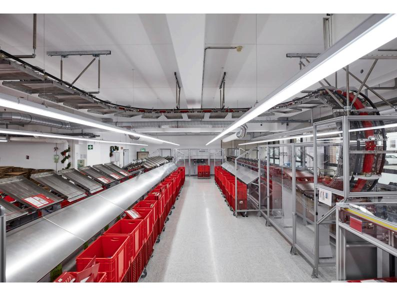
Denisort is an innovative tilt-tray sorter that combines conveying, order picking and sorting in one seamless and scalable system with universal applications across a wide range of intra-logistic processes. The basis is a carrier chain that runs energy-efficiently and quietly on low-friction rollers in a steel profile. The system thus enables individual solutions with a completely free layout in all dimensions, even across several levels.
